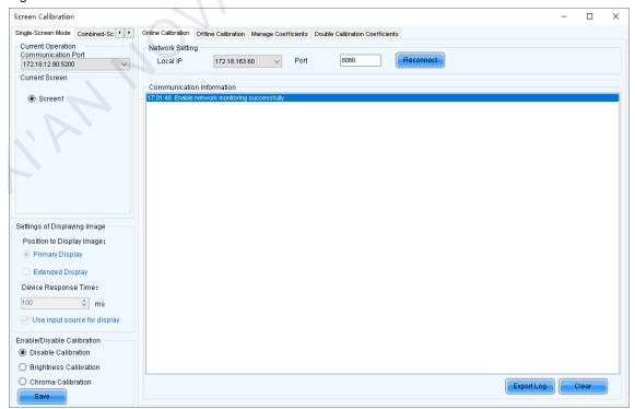
Step 3 Select the Single-Screen Mode tab or Combined-Screen Mode tab.
