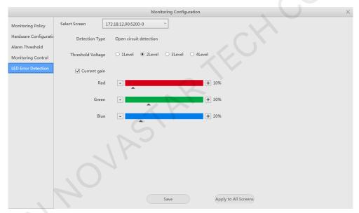
Set the LED error detection parameters. After the settings are done, click Save or Apply to All Screens.
