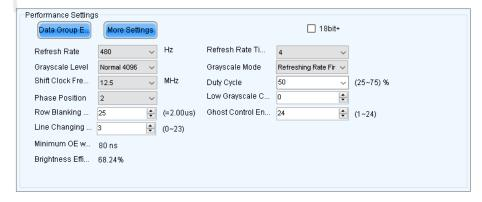
The performance parameters displayed in the area varies depending on the receiving card. The main parameters include the followings.
