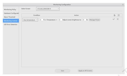
Set the rules for automatic control of average temperature, maximum temperature, smoke and backup power supply. If the control type is set to smoke, a multifunction card must be configured in advance. After the settings are done, click **Save** or **Apply to All Screens**.
