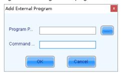
Step 3 Select the program path and enter the command line parameter as required, and then click **OK**.
