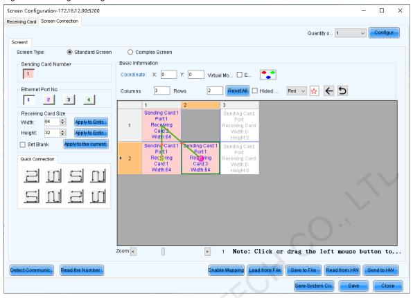
Step 7 Repeat Step 4 to Step 6 to set the receiving cards loaded by the other output ports.
