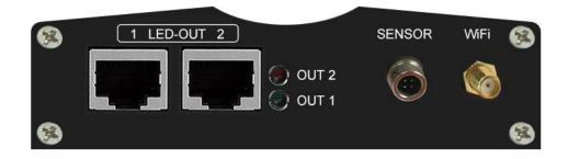
【1 LED-OUT 2】 It is used for connecting gigabit net-port of the receive controller.
