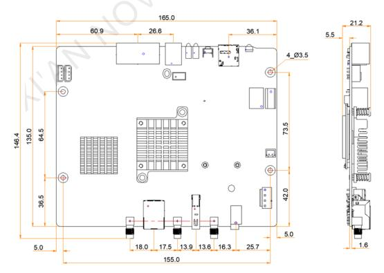
If you want to make molds or trepan mounting holes, please contact NovaStar for structural drawings with higher precision.
