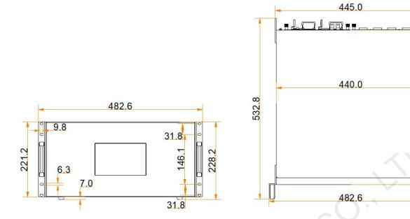
Tolerance: ±0.5 Unit: mm
