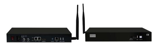
C6 supports U disc plug and play, fully compatible with the edition and play mode under synchronized play system. It is needed just for one press to send the programs into the U disc to play it. Also it is available for program updates and management through wire network.
